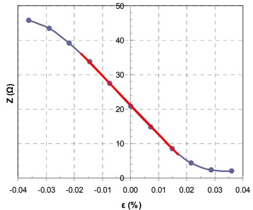
Figure 3. Dependence of HSSG impedance on the applied stress,  $\epsilon = \Delta l/l$
