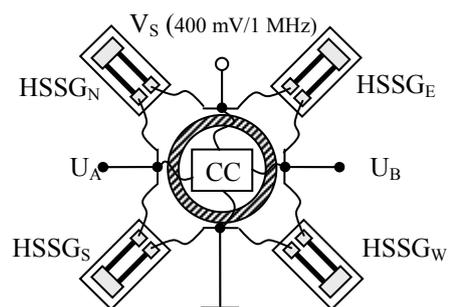
Figure 4. Schematic of a strain bridge: HSSG<sub>N,S,E,W</sub> - Strain gauges mounted along the N, S, E and W directions, CC - conditioning circuitry
