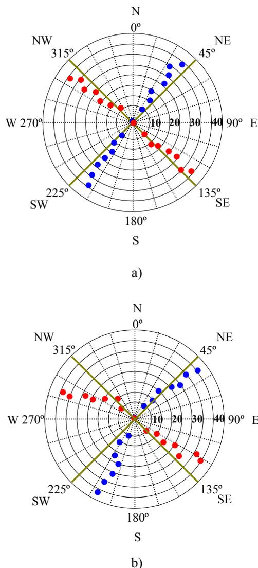
Figure 9. Representation in polar coordinates of the displacement amplitude and angle direction calculated with equations (1) and (2) in the two arrangements of Fig. 7 and Fig. 8.
