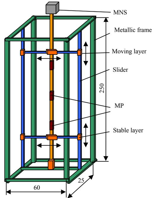
Figure 6. Schematic representation of the experimental setup. Dimensions are in cm.
