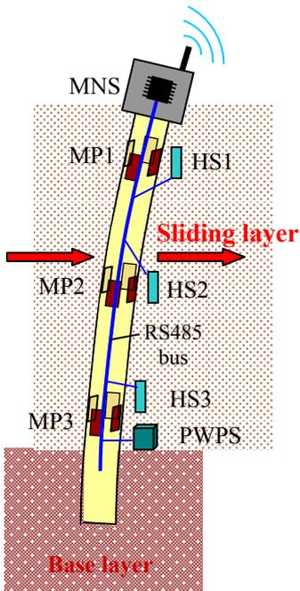
Figure 1. The MN structure: MNS - measurement node server, MP - measurement points, HS - humidity sensor, PWPS - pore water pressure sensor
