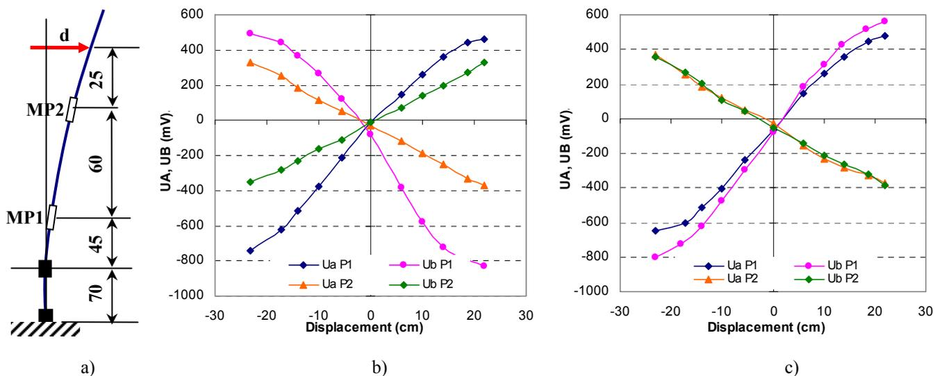
Figure 7. Representation of the voltages delivered by two measurement points vs. displacement  $d$  of the mobile fulcrum: a) particular emplacement of MPs with respect to fixed and mobile fulcrums, b) representation  $U_{A,B} = f(d)$  for NE-SW orientation of displacement, c) representation  $U_{A,B} = f(d)$  for NW-SE orientation of displacement.
