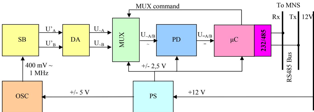
Figure 5. Block diagram of the signal conditioning circuitry for a measurement point: SB - strain bridge, DA - differential amplifier, OSC - sinusoidal oscillator, MUX - analog multiplexer, PD - peak detector, PS - power supply,  $\mu C$  - microcontroller
