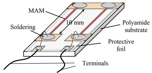
Figure 2. Structure of a highly sensitive strain gauge (HSSG)
