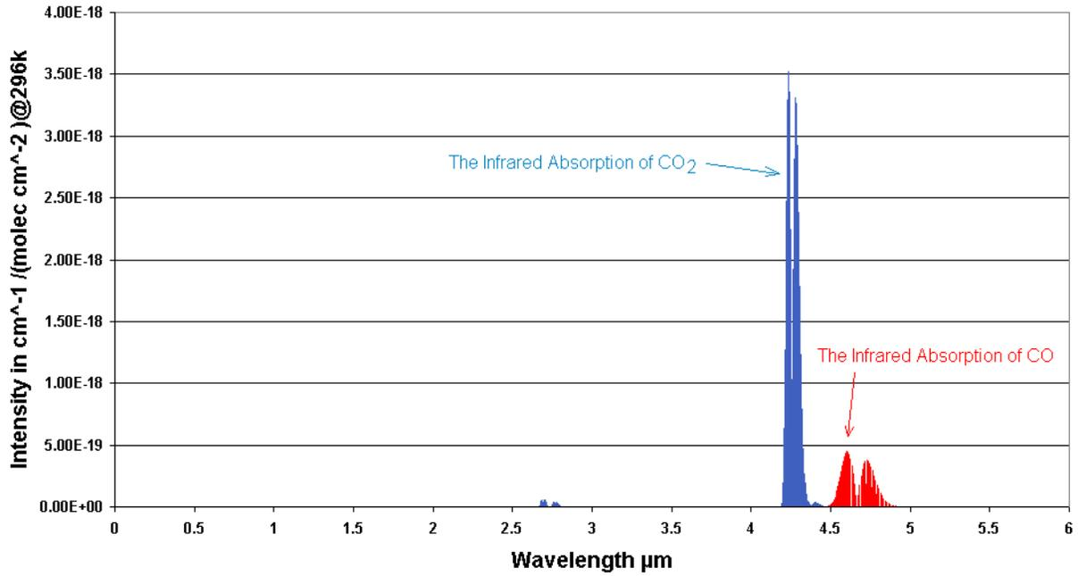
Figure 1 Theoretical Absorption Spectra for CO and CO<sub>2</sub> gases [3]
