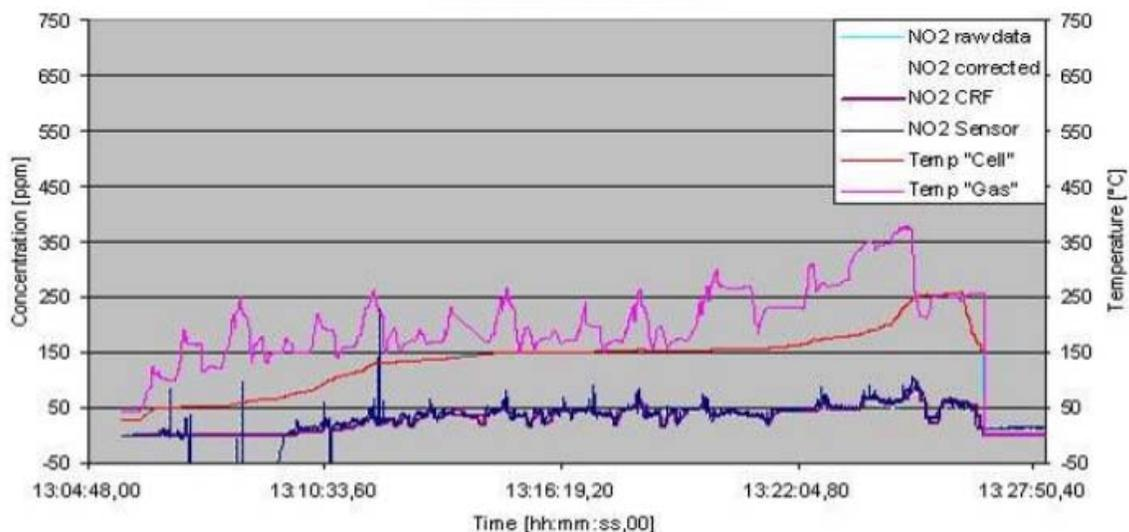
Figure 9.  $\text{NO}_2$  Test Results Under the Car With Simultaneous Reference Instruments Recording
