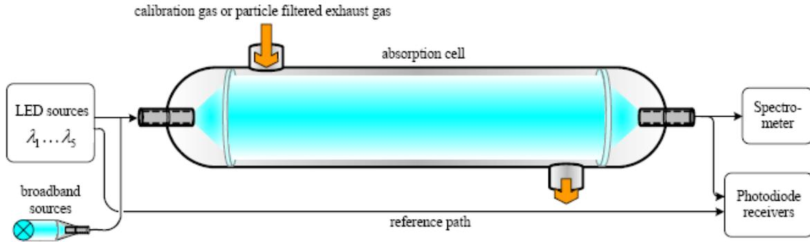
Figure 7 The Gas Sensor for Measuring in Ultra Violet Range
