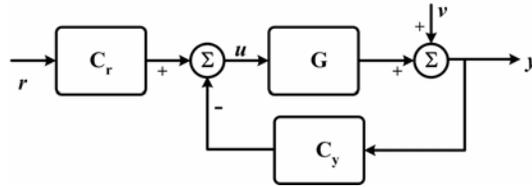
Fig. 1: Block diagram of 2-DOF controller
