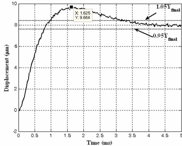
Fig. 5: Simulation with nominal PID controller
