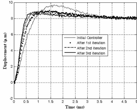
Fig. 6: Tuning of PID controller using IFT (Simulation)
