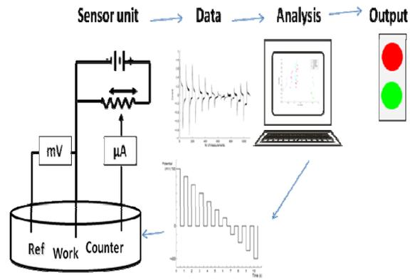
Figure 6: The concept of the electronic tongue system
