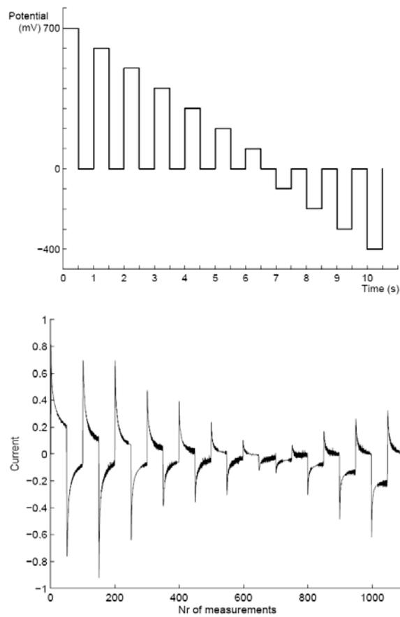
Figure 7. The electronic tongue sensor input (upper figure) and response (lower figure).
