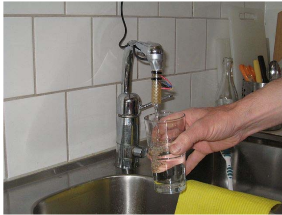
Figure 5. The electronic tongue device on the water tap
