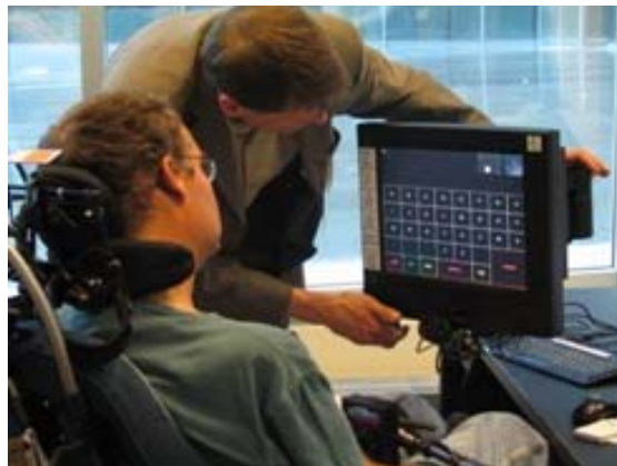
Figure 4: Gaze detection pointing system for people with disabilities (taken from www.adamfulton.co.uk )
