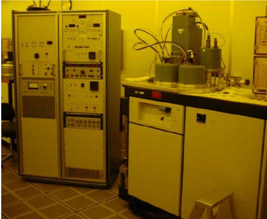
Figure 1. Sputter deposition system. This system is capable of depositing on substrates, which are as large as 6 inches. This system is cryo-pumped with a base pressure measured at 1.1 \times 10^{-7} torr.
