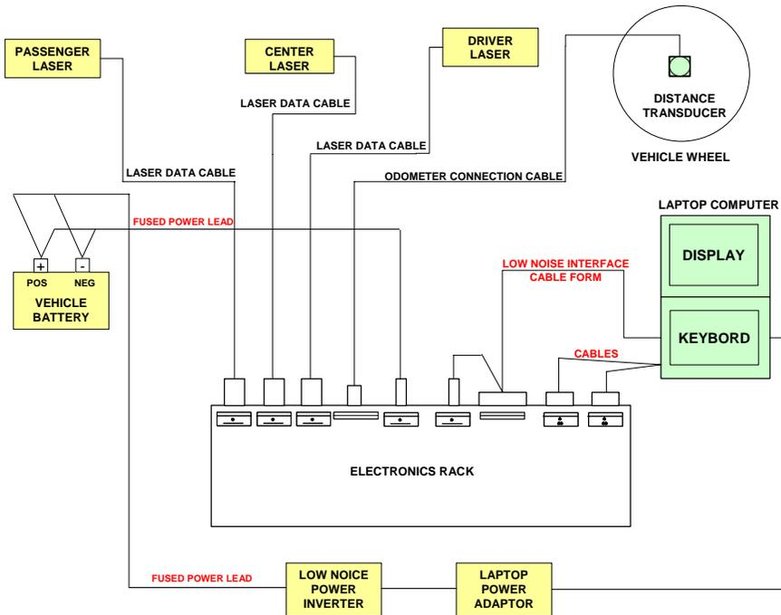
Figure 5. Outline of Laser Profiler System
