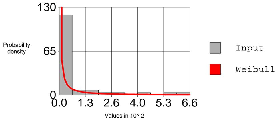
Figure 10. Weibull distribution of the two periods' slope differences (right wheel path)
