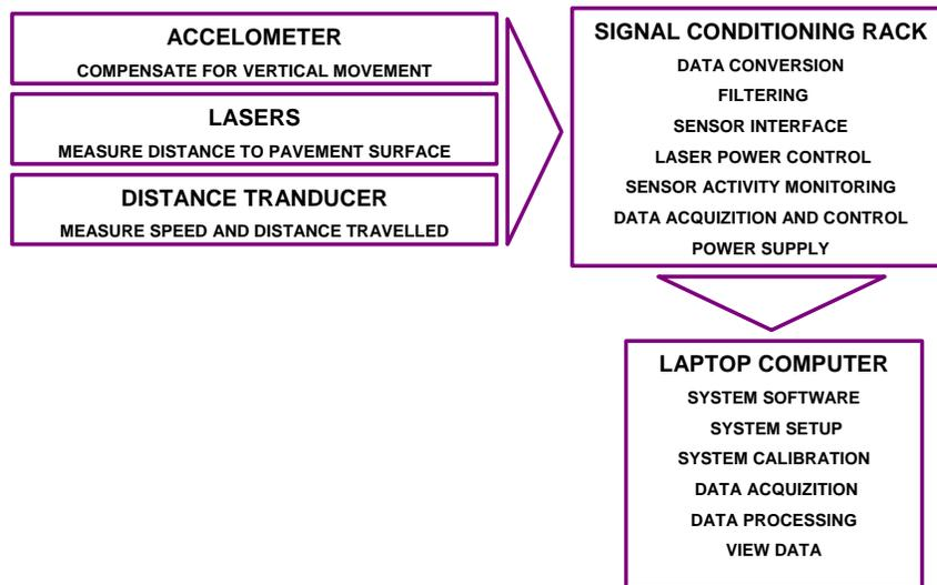
Figure 4. Laser Profiler block diagram
