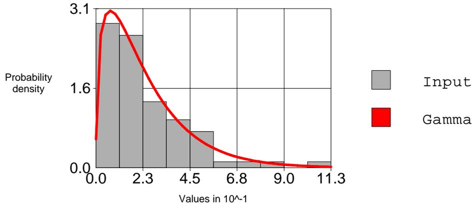
Figure 8. Gamma distribution of the two periods' IRI absolute differences (right wheel path)
