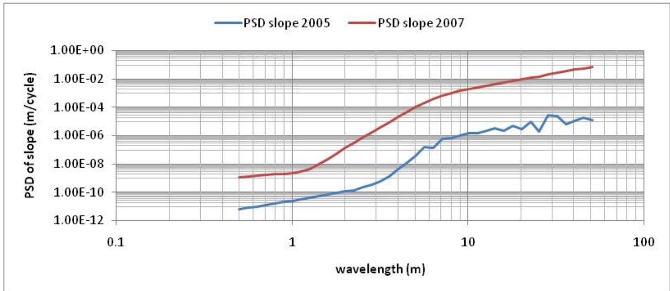
Figure 9. PSD slopes of the two periods' sensed profile (right wheel path)
