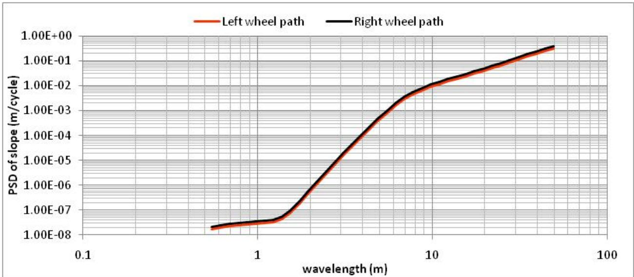
Figure 3. PSD of slope (wavelengths 0.5-50 m)
