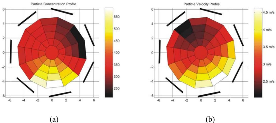
Figure 3. (a): Reconstructed particle velocity profile and (b): Reconstructed relative particle concentration profile for dilute phase flow of plastic pellets [30].
