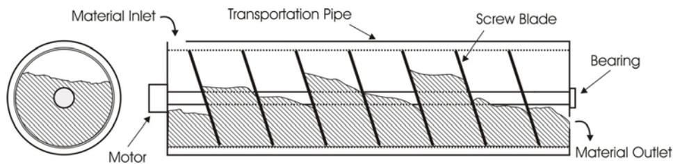
Figure 4. Material transportation through a screw conveyor showing different fill levels [32].
