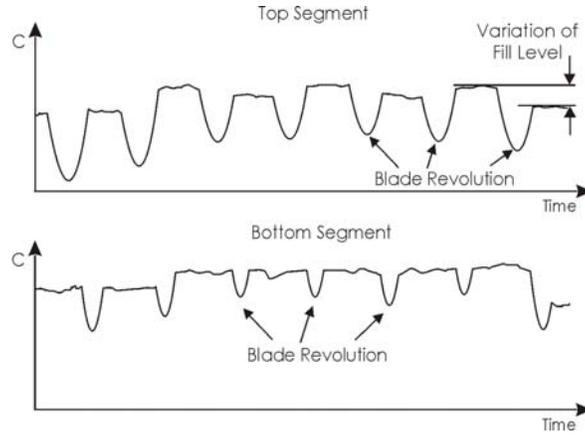
Figure 5. Principle of operation of the screw conveyor flow meter to determine revolution speed of the screw and material fill level.
