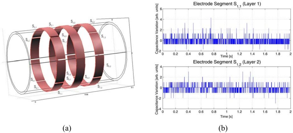
Figure 1. (a): Topology of the sensor front-end with two segmented transmitter layers and one common receiver ring in-between and (b): Measurement results for two corresponding segments in dilute phase flow [30].
