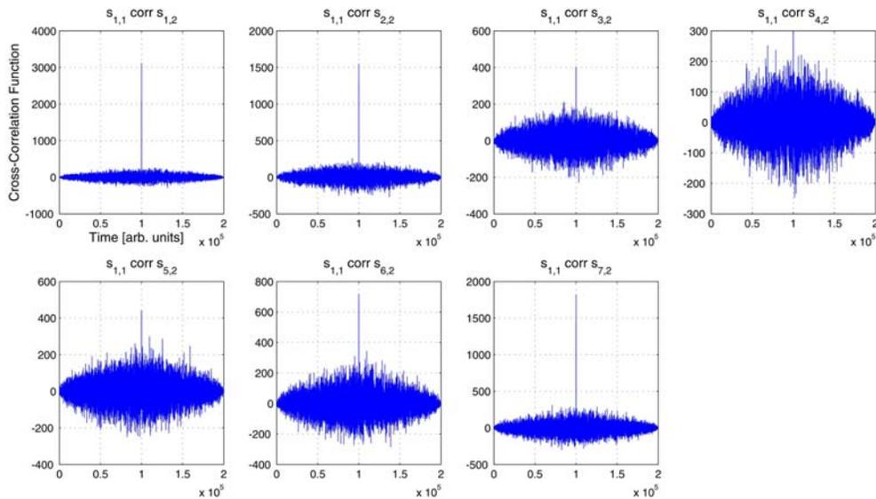
Figure 2. Cross-correlation functions of a signal of segment  $S_{1,1}$  and all other segment signals of layer 2 [30].
