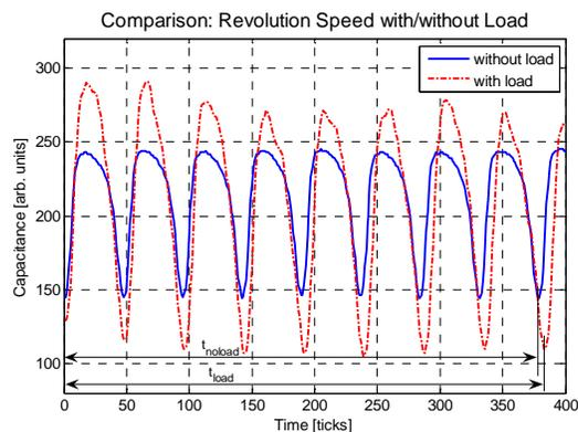
Figure 8. Bottom segment signal when the screw conveyor is operated with dry corn (with load, dashed-dotted red line) and without load (solid blue line).
