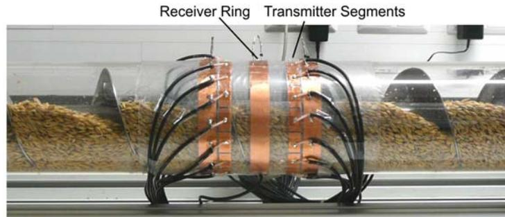
Figure 6. Setup of the capacitive flow sensor mounted on a non-conductive screw conveyor pipe.
