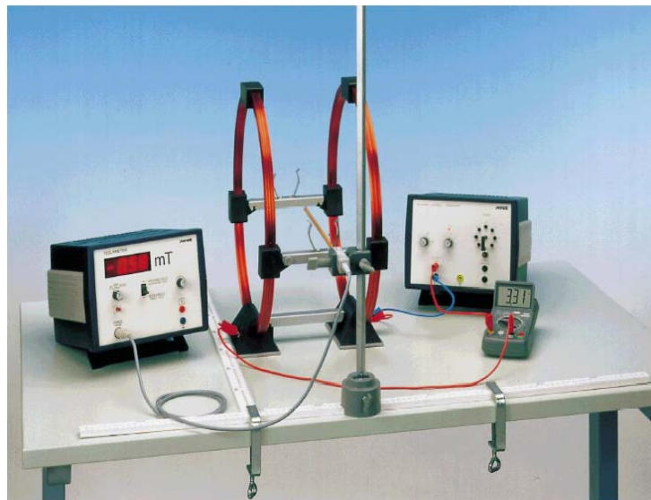
Fig. 12. The experimental set-up of Helmmoltz coil
