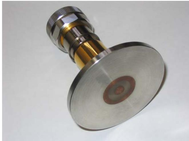
Figure 1. Coaxial probe fabricated from air line.
