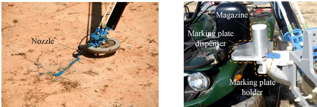
Figure 4: Paint marker and marking plate dispenser.
