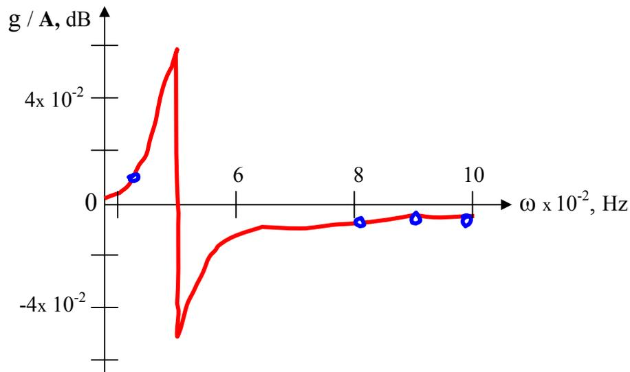
Fig. 5. Calculated amplitude-frequency characteristic of the MTMQ: the circles represent the experiment data [12]. The  $\mathbf{A}$  is a response of the MTMQ.
