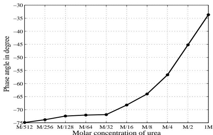
Figure 14. The CPA reading of the sensor at different concentration of Urea solutions. The readings are taken at 100 kHz in the CPA zone.
