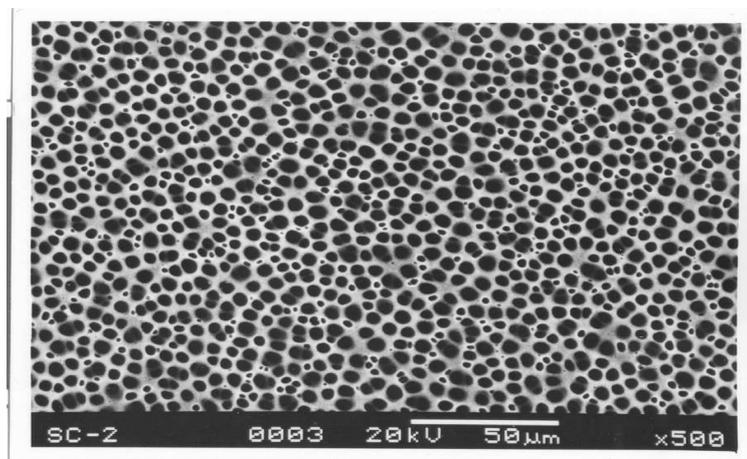
Figure 5. Porous surface of the electrode after coating: coating thickness is  $12\ \mu\text{m}$ . Diameter of the pore is about  $5\ \mu\text{m}$ .
