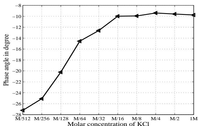
Figure 12. The CPA reading of the sensor at different concentration of KCl solutions. The readings are taken at 100 kHz in the CPA zone.
