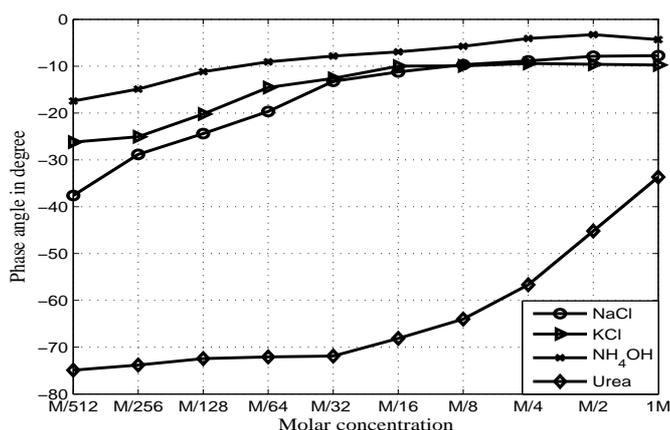
Figure 15. Comparison of responses between NaCl, KCl, NH<sub>4</sub>OH and Urea solution at different molar concentration.
