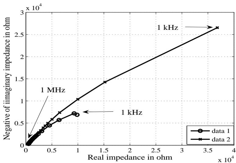
Figure 10. Real versus imaginary impedance plot in 9.2 pH solution, data 1: porous electrode with  $5\mu\text{m}$  coating thickness, data 2: porous electrode with  $12\mu\text{m}$  coating thickness.
