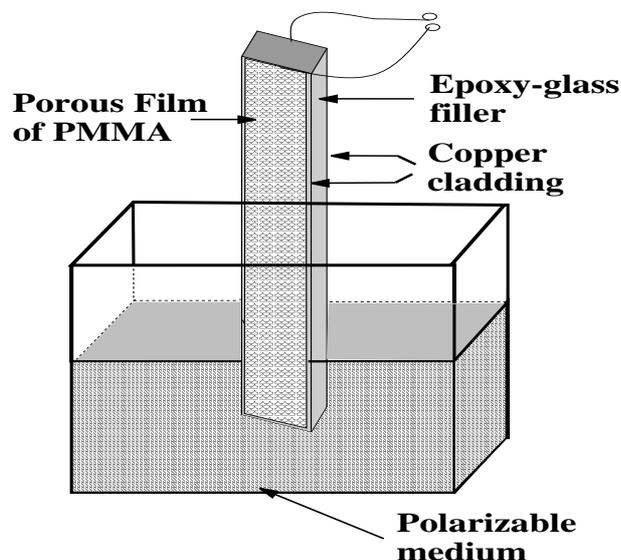
Figure 2. Construction of the CPE with microporous-PMMA-film coated electrode.
