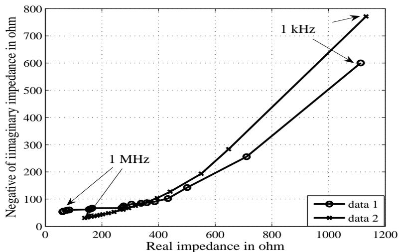
Figure 8. Real versus Imaginary impedance plot in 1M KCl, data 1: porous electrode with  $5\mu$  coating thickness, data 2: porous electrode with  $12\mu\text{m}$  coating thickness.
