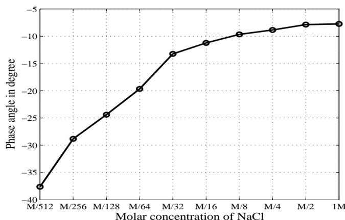
Figure 11. The CPA reading of the sensor at different concentration of NaCl solutions. The readings are taken at 100 kHz in the CPA zone.
