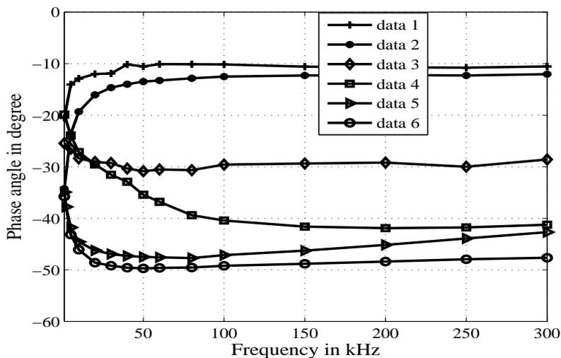
Figure 7. CPA behaviour obtained for two different porosity, data 1,2: 1M KCl, data 3,4: tap water (conductivity =  $239\mu\text{mho/cm}$ ), data 5,6: 9.2 pH. Data 1, data 3 and data 5 are for bigger pore ( $5\mu\text{m}$  coating thickness); data 2, data 4 and data 6 are for smaller pore ( $12\mu\text{m}$  coating thickness).
