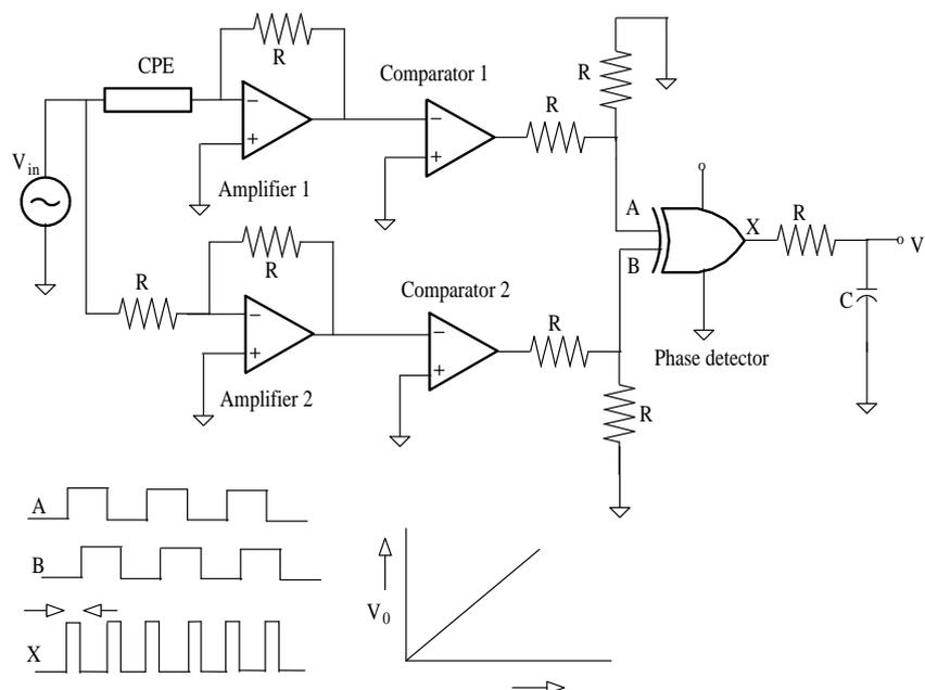
Figure 16. The phase angle detector circuit which gives the output in voltage with the phase angle input.
