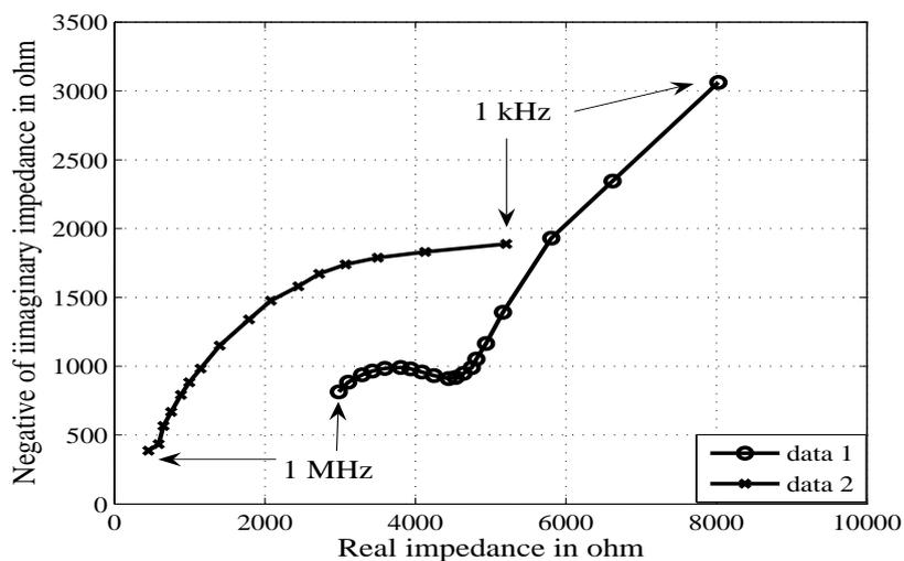
Figure 9. Real versus imaginary impedance plot in tap-water (conductivity =  $239\mu\text{mho/cm}$ ), data 1: porous electrode with  $5\mu\text{m}$  coating thickness, data 2: porous electrode with  $12\mu\text{m}$  coating thickness.
