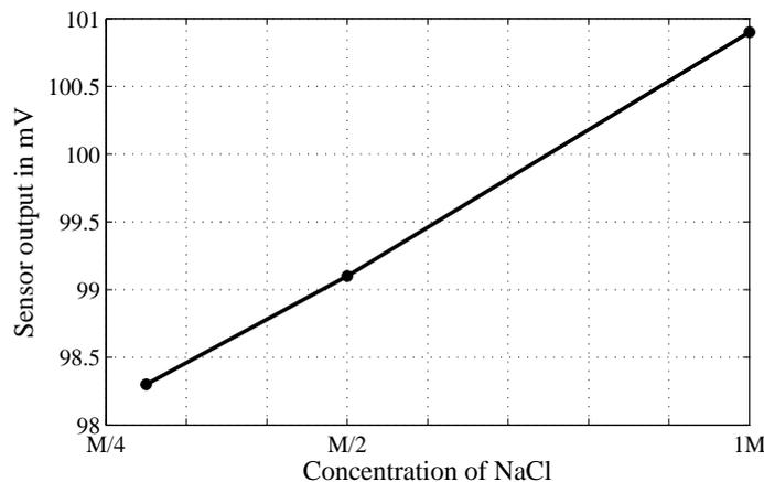
Figure 18. The performance of the CPE sensor in different concentrations of NaCl solutions
