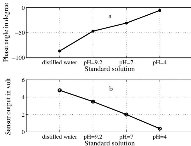
Figure 17. The performance of the CPE sensor in distilled water and three different pH solutions. (a) the value of the constant phase angle at different standard solutions, (b) The output voltage obtained from the detector circuit
