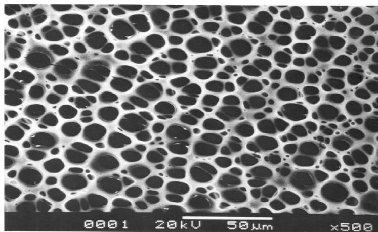
Figure 4. Porous surface of the electrode after coating; coating thickness is 5 μm. Diameter of the pore is about 10 μm.
