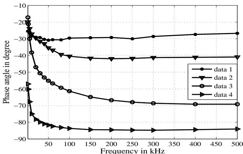
Figure 6. The CPA behaviour of four different CPE with different coating thickness. Data 1: 5  $\mu\text{m}$  coating thickness, data 2: 12  $\mu\text{m}$  coating thickness, data 3: 28  $\mu\text{m}$  coating thickness, data 4: 47  $\mu\text{m}$  coating thickness. The probe is dipped in tapwater.
