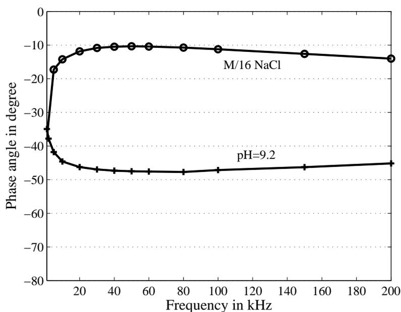
Figure 1. The CPA in the aqueous solution of pH=9.2 and in 1/16 molar NaCl solution.
