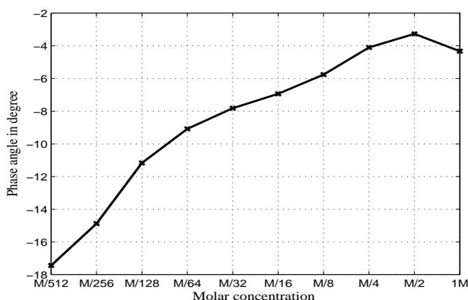
Figure 13. The CPA reading of the sensor at different concentration of  $\text{NH}_4\text{OH}$  solutions. The readings are taken at 100 kHz in the CPA zone.
