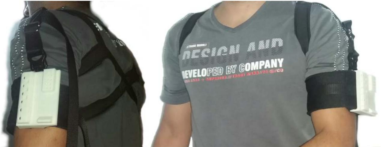
Figure 4: Attachment system to fix the exoskeleton to the body of the user.
