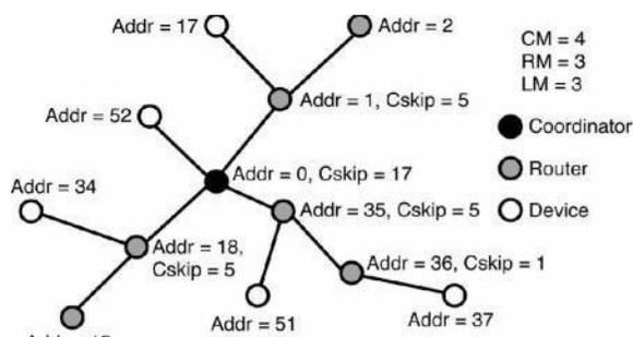
**Fig1** ZigBee Cluster Tree
