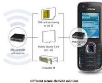
Fig.1: Communication among NFC controller and mobile phone
