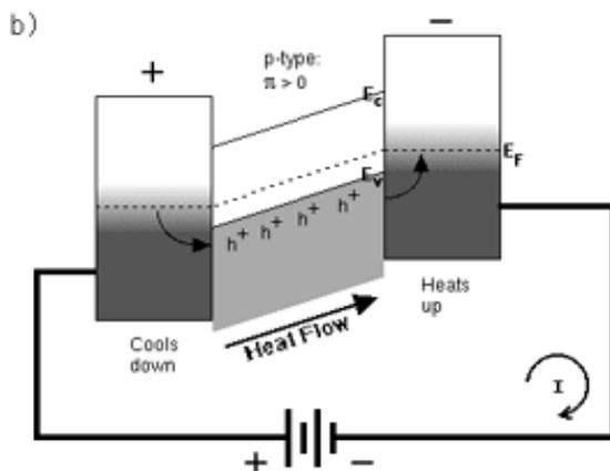
Fig4.  $\Pi > 0$ ; Positive Peltier coefficient
