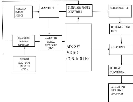
Fig6. Block diagram of hybrid power converter
