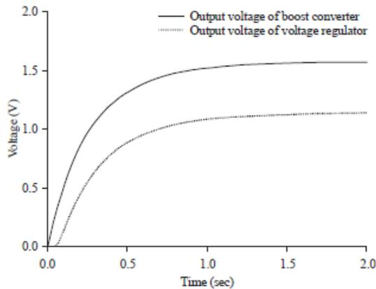
Fig6. Performance of harvester using thermal energy
