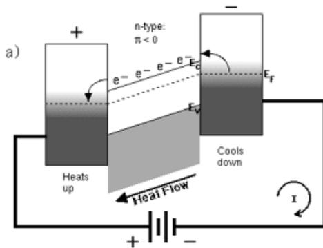
Fig3.  $\Pi < 0$  ; Negative Peltier coefficient
