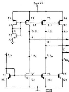
FIGURE 4.1. CIRCUIT OF SIMPLE CURRENT COMPARATOR IN TRI STATE
