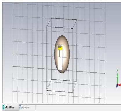
**Fig.15. Mobile patch antenna interaction with head model**
