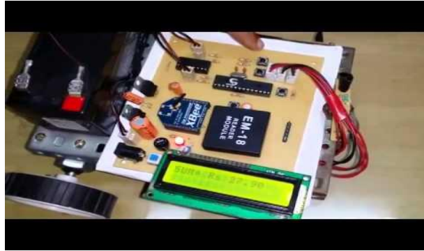
Fig 6- Overview of RFID kit
