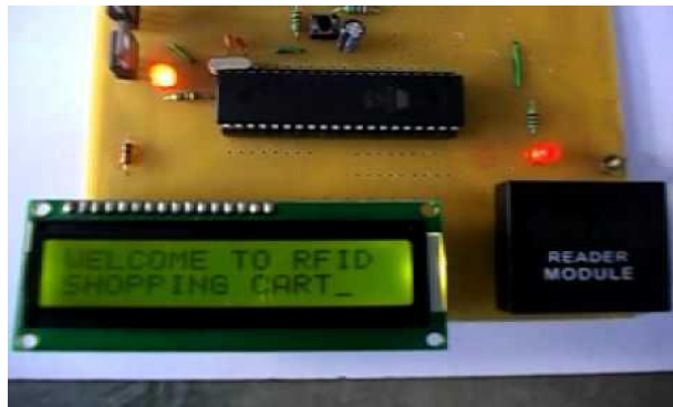
Fig 4- RFID shopping cart kit
