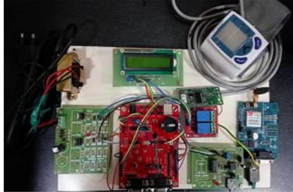
Figure.11 Interfacing of BP sensor and GPRS module
