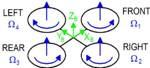
Fig [2] – quadcopter structure model in hovering condition
