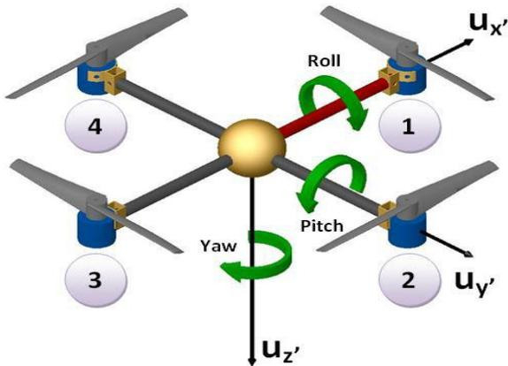
Figure [3] – yaw ,pitch and roll movements of quadcopter
