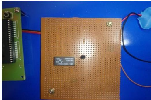
Fig.14 Relay Circuit
