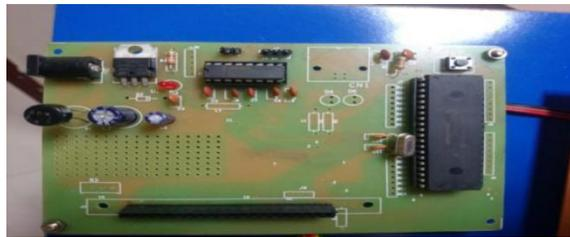
Figure 13 shows the overview of PIC microcontroller along with the interface board for LCD display.
