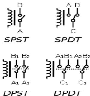
Fig.4 Circuit diagram of relays
