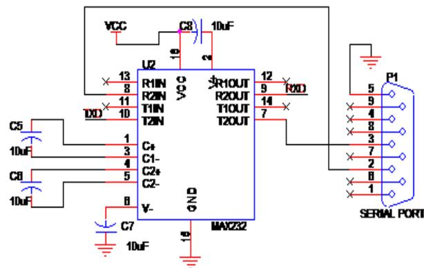
Fig.3 Circuit diagram of RS232 to TTL converter
