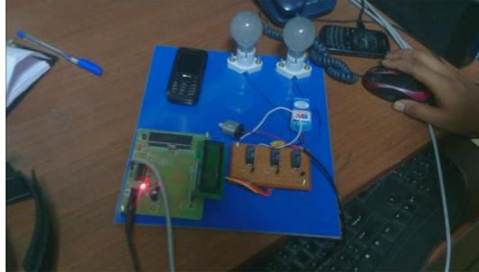
Fig.16 PIC Controller and Relay Circuit with connected Devices.
