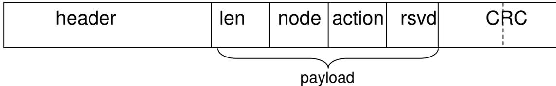
Figure 7. Custom Message Structure for Over the Air Programming
