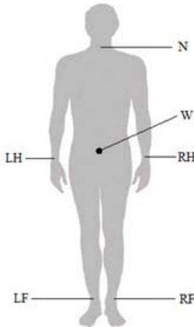
Figure 3. Tri-axial Accelerator Sensors Position
