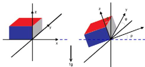
Figure 4. Tri-axial angle
