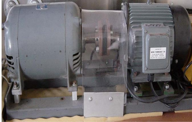
Figure 8: The experimental set-up of motor and dynamometer
