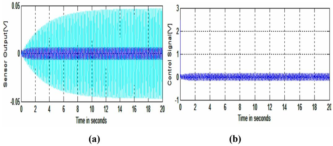
Figure 3 Response to excitation at first natural frequency with simultaneous POF for lower bound system
