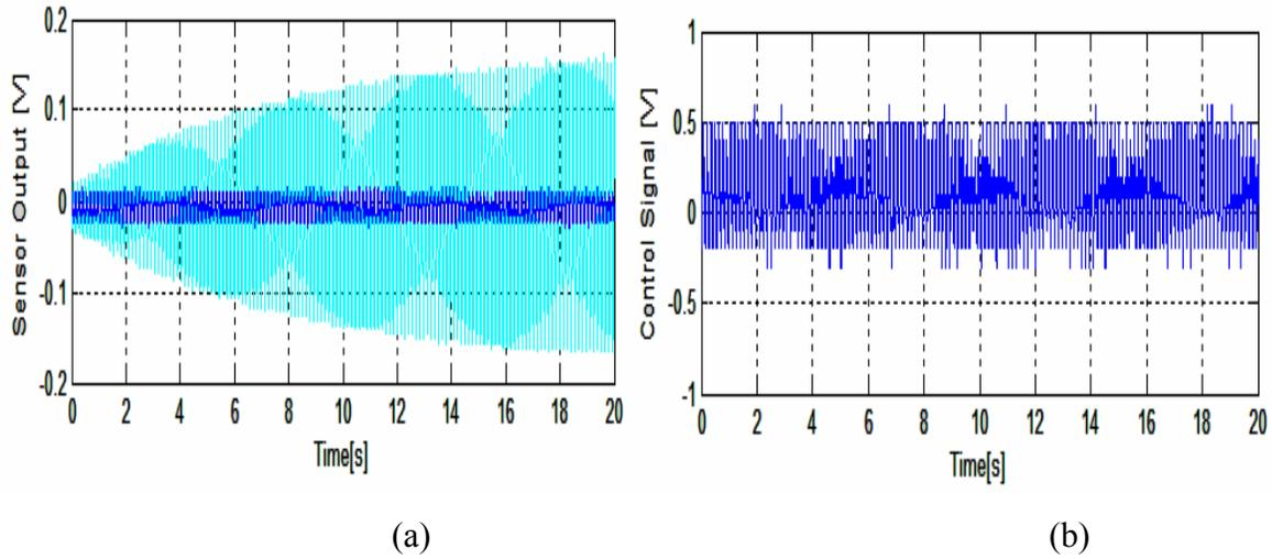
Figure 6. Response to excitation at first natural frequency for the nominal system
