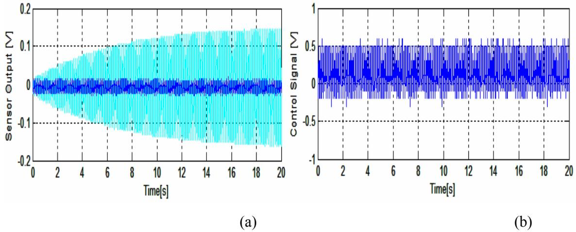
Figure 8. Response to excitation at first natural frequency with decreased in beam length ( Experimental)
