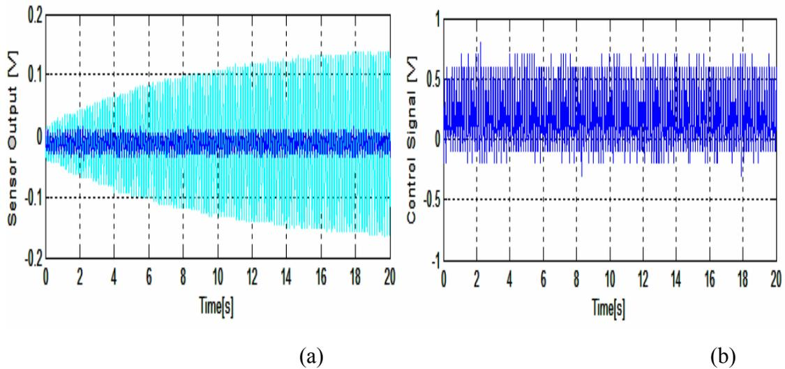
Figure 7. Response to excitation at first natural frequency with increased in beam length
