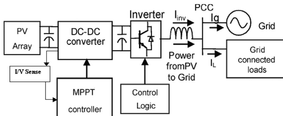
**Figure 3: System configuration for grid connected PV-based system**
