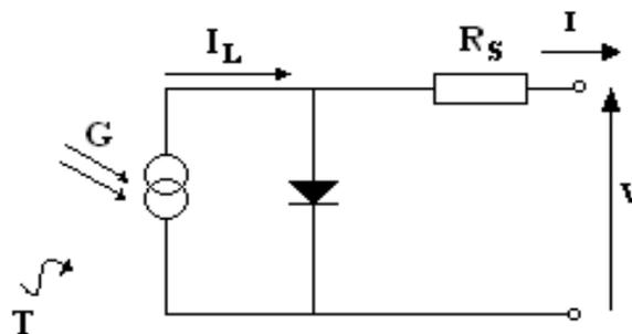
**Figure 2. Circuit model of a PV cell**
