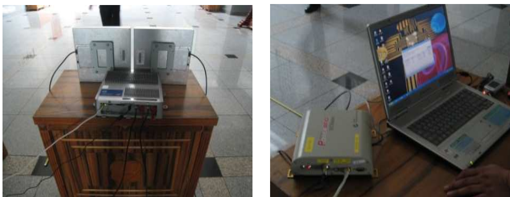
Figure 15. 900 MHz RFID Tag License Plates Test Device
