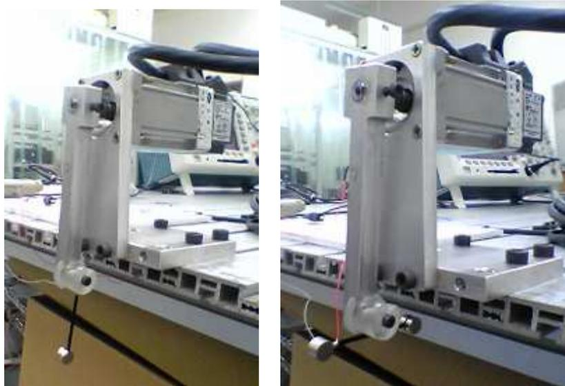
Figure 6. Cantilever type (left) and airfoil type (right) piezoelectric generators attached to swing arm
