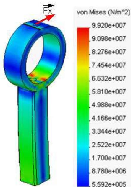
Figure 4. Stress result of  $F_x$  shearing force
