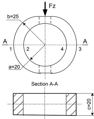
Figure 2. The cross section of the proving ring
