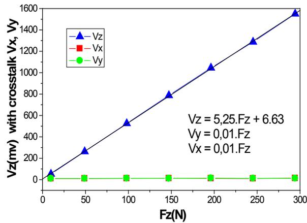
Figure 13. Results of the  $F_Z$  force calibration
