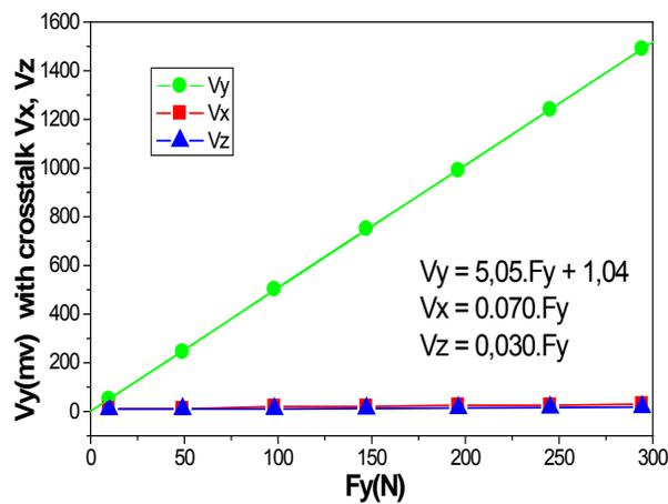
Figure 12. Results of the  $F_y$  force calibration
