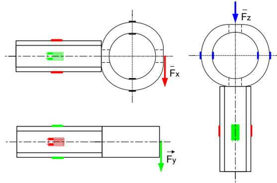
Figure 10. A 3D Sensor position for calibration
