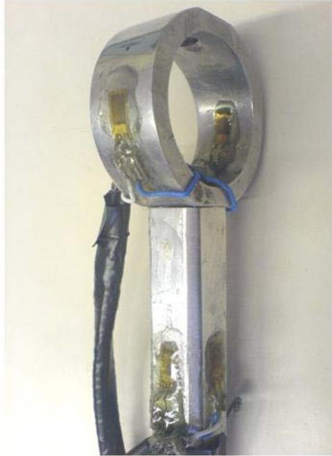
Figure 7. The 3D force sensor realization
