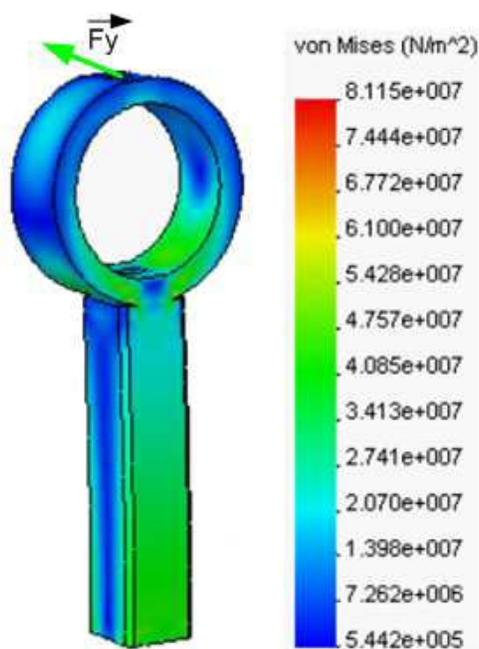
Figure 5. Stress result of  $F_y$  shearing force
