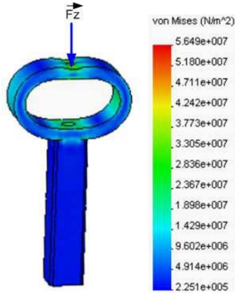
Figure 6. Stress result of  $F_z$  comprising force
