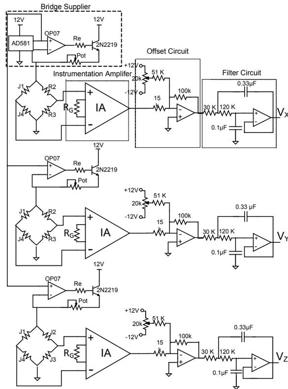
Figure 8. The conditioning Circuit
