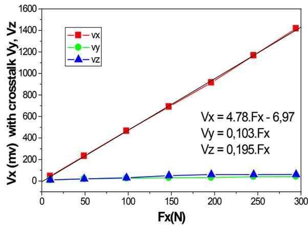
Figure 11. Results of the  $F_x$  force calibration
