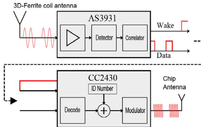
Figure 5. Block diagram of the receiving system.
