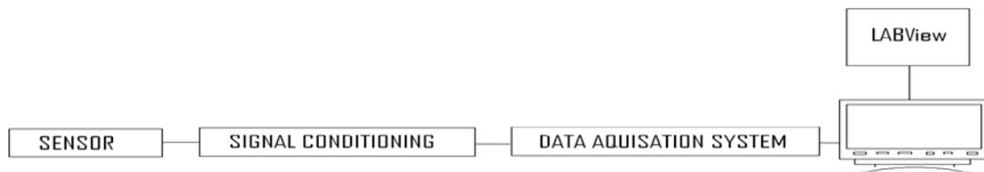
Figure 1: Sensor characterization block diagram
