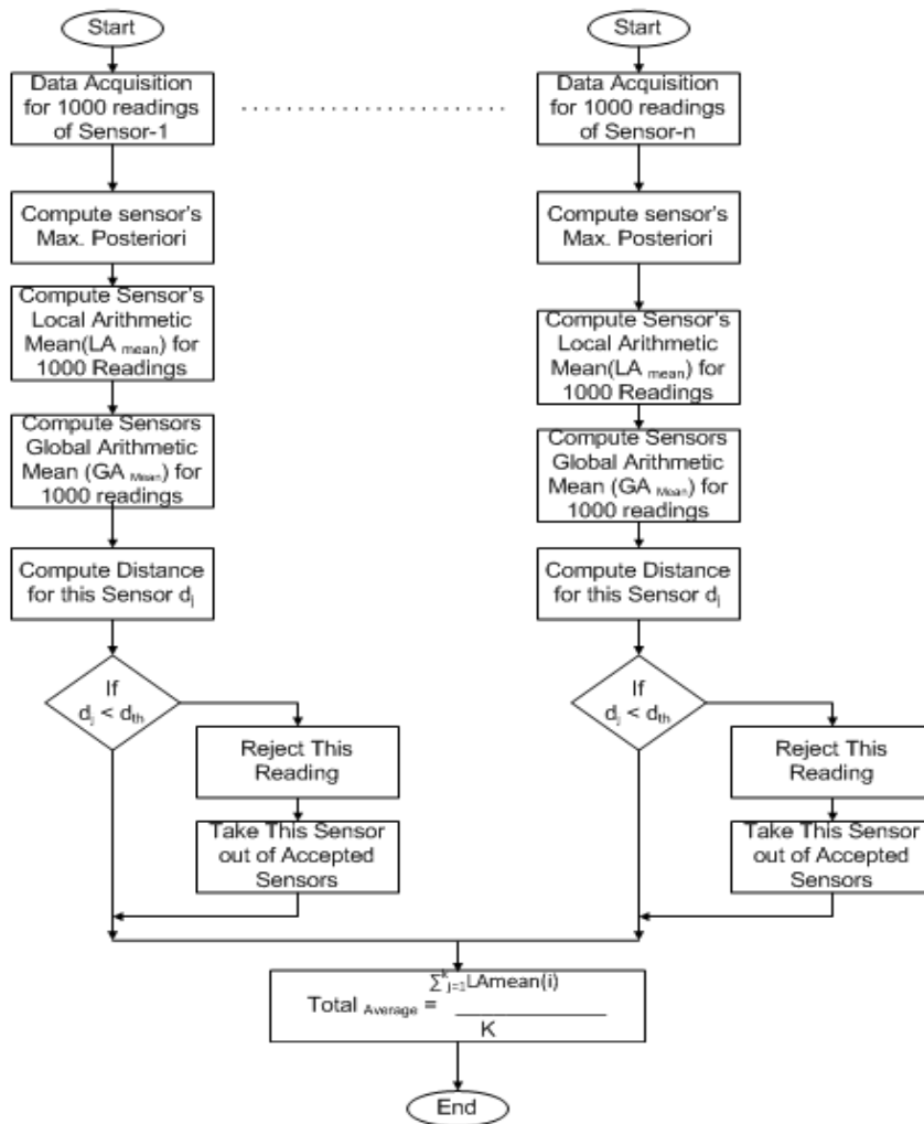
Figure 4. Flow chart shows how sensor similarity is performed.
