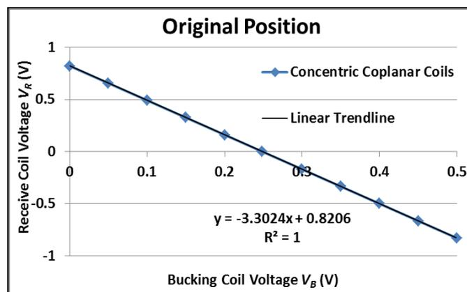
Figure 5:  $V_R$  vs  $V_B$  for concentric coils
