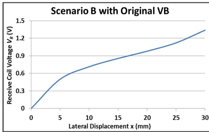
Figure 12:  $V_R$  vs  $x$  for Scenario 'B',  $V_B$  constant
