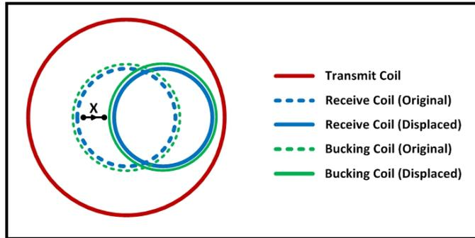
Figure 6: Displacement, receive coil concentric with bucking
