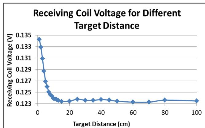
Figure 13:  $V_R$  vs target distance  $z$  for gold ring target
