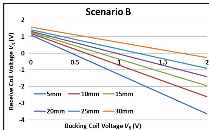
Figure 10:  $V_R$  vs  $V_B$  for bucking coil concentric with transmit
