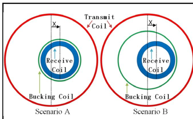
Figure 2: Scenarios A and B for coil displacement
