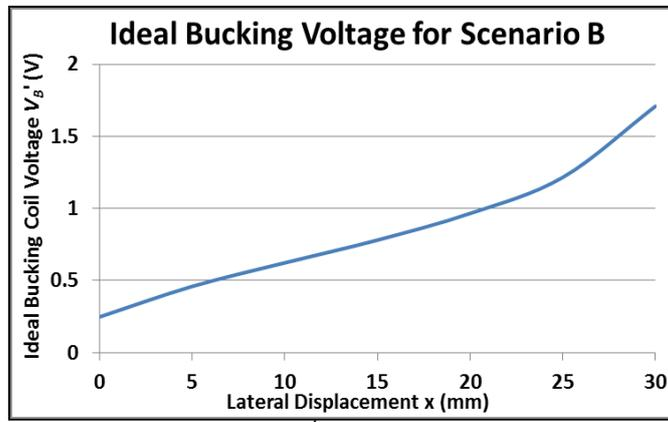
Figure 11:  $V_B$  vs  $x$  for Scenario 'B'
