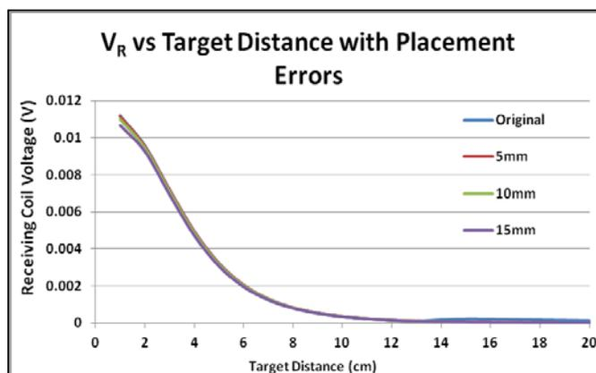
Figure 14:  $V_R$  vs target distance for 0 to 15 mm head offset
