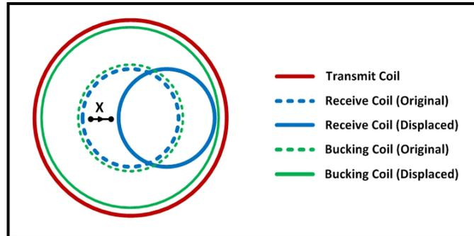
Figure 9: Displacement, bucking coil concentric with transmit
