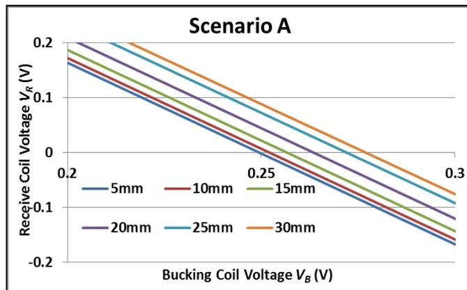
Figure 7:  $V_R$  vs  $V_B$  for receive coil concentric with bucking
