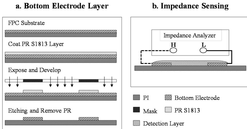
Figure 4: Microfabrication process of PANDB sensor
