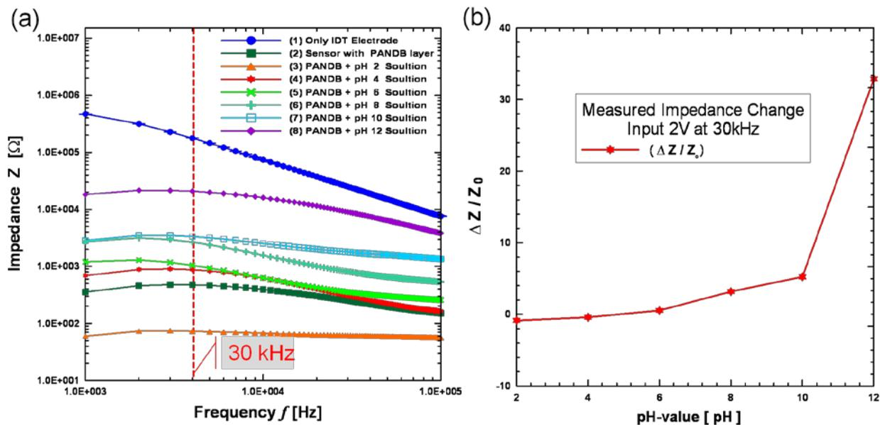
Figure9: Impedance measurement from pH2 to pH12
