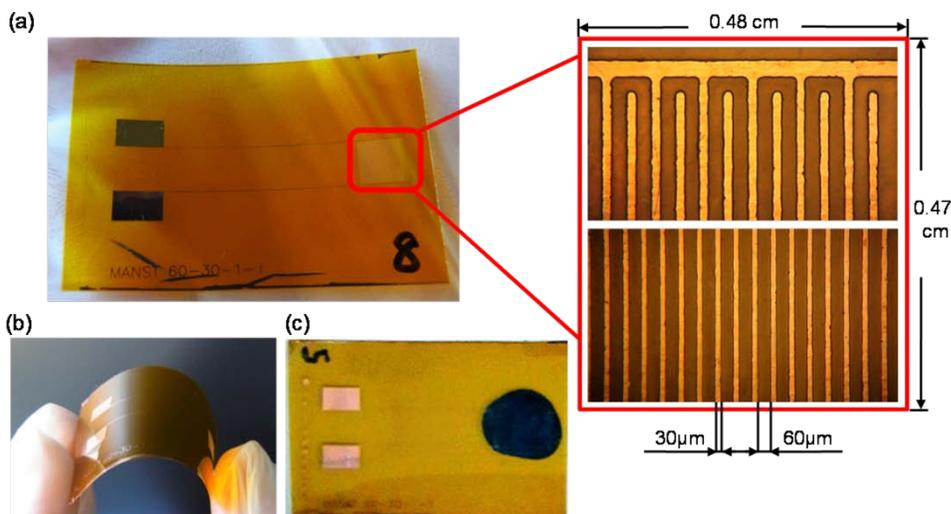
Figure 5: (a) IDT electrode array on FPC, and optical micrograph of IDT electrodes; (b) bendable sensor; (c) finished flexible pH value sensor with PANDB layer within IDT electrode array
