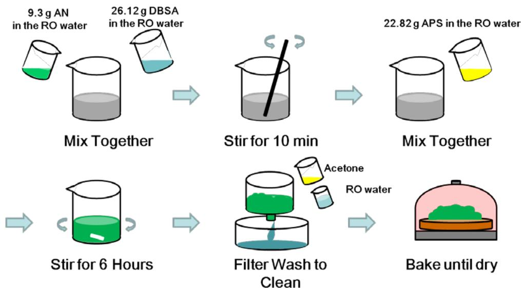
Figure 3: Scheme of the synthesis process of PANDB
