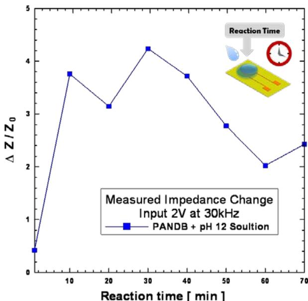
Figure 7: Normalized impedance change for different reaction times.
