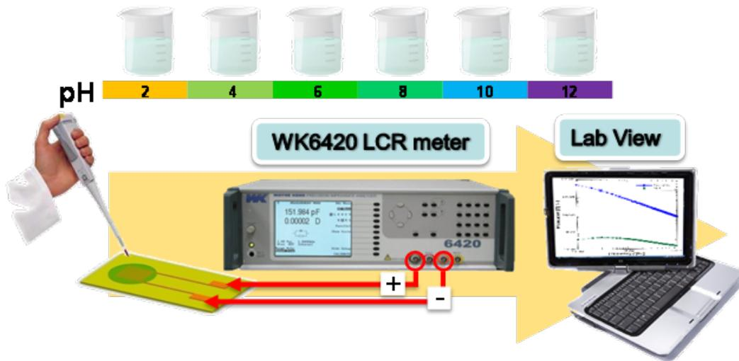
Figure 6: Experimental setup and impedance sensing of different pH solutions
