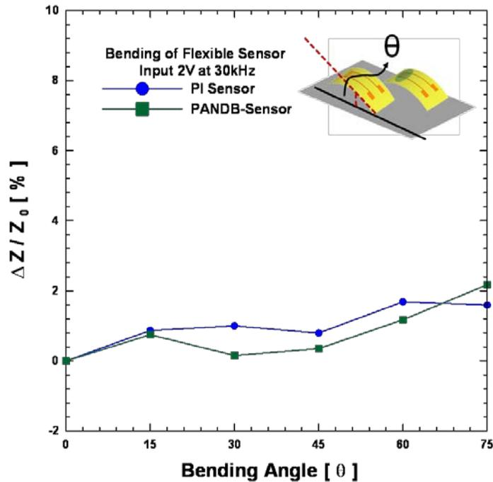
Figure 10: Flexibility of sensor
