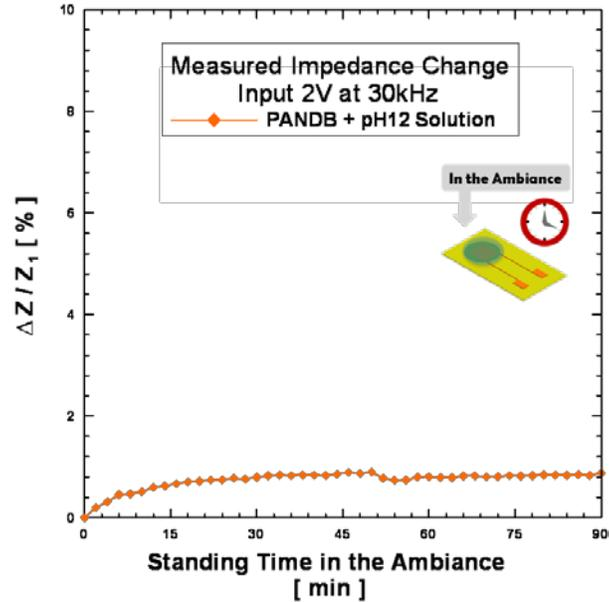
Figure 8: Impedance variation at room temperature within 90 min
