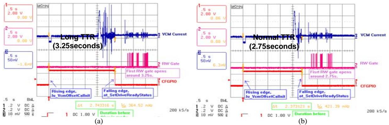
Figure 7. TTR Comparison for drive operating at cold temperature:
