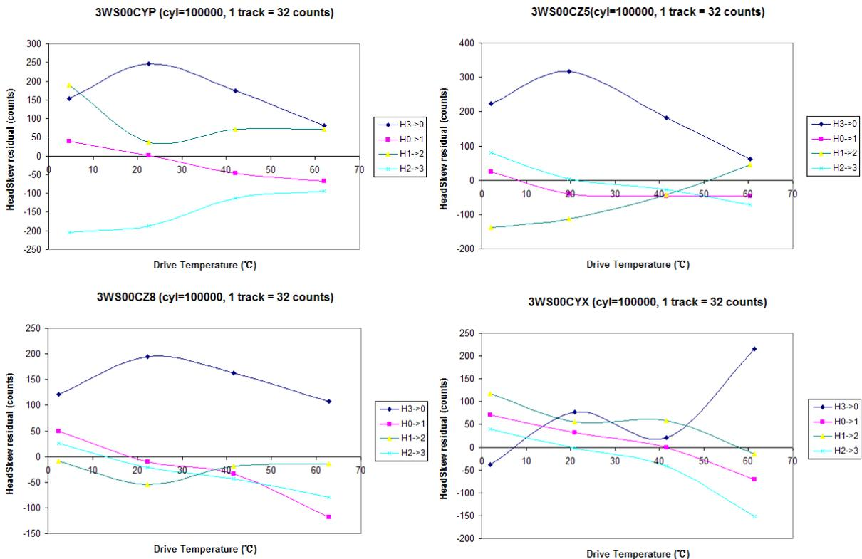
Figure 6. Head skew residual with temperature compensation
