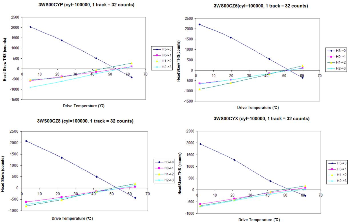
Figure 5. Head skew deviation against drive temperature
