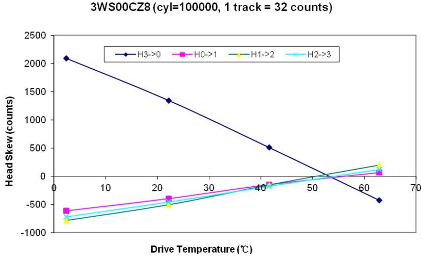
Figure 3. Temperature-induce head skew variation
