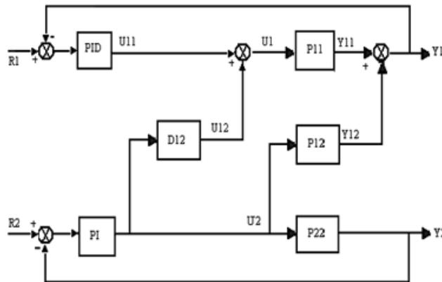
Figure 9: A partial decoupling control system
