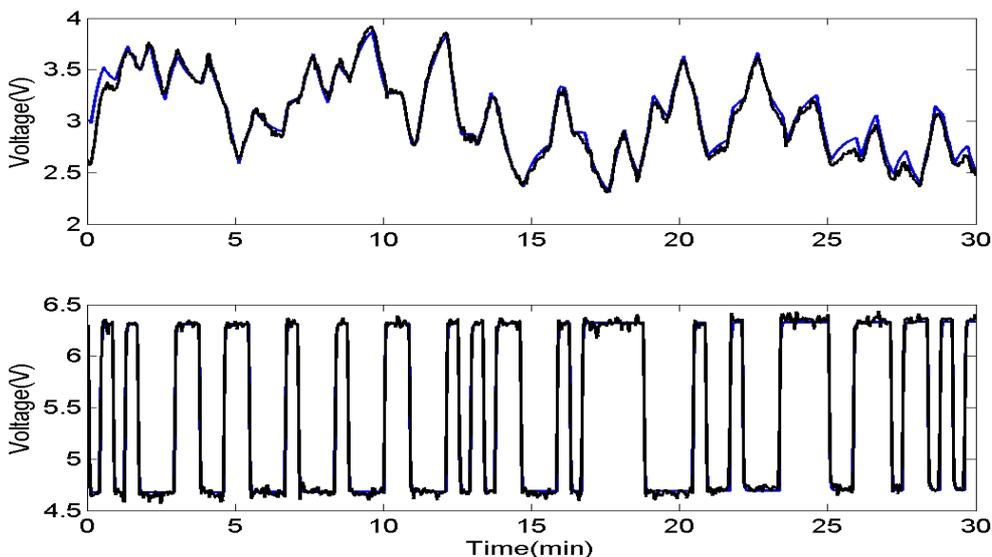
Figure 7: Cross-validation results (black: measured output; blue: simulated output)
