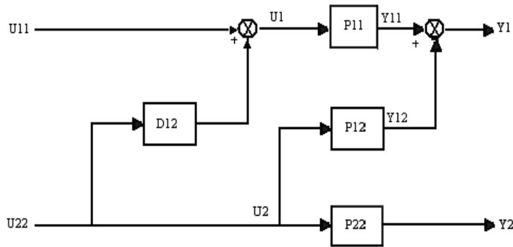
Figure 8: Decoupled system
