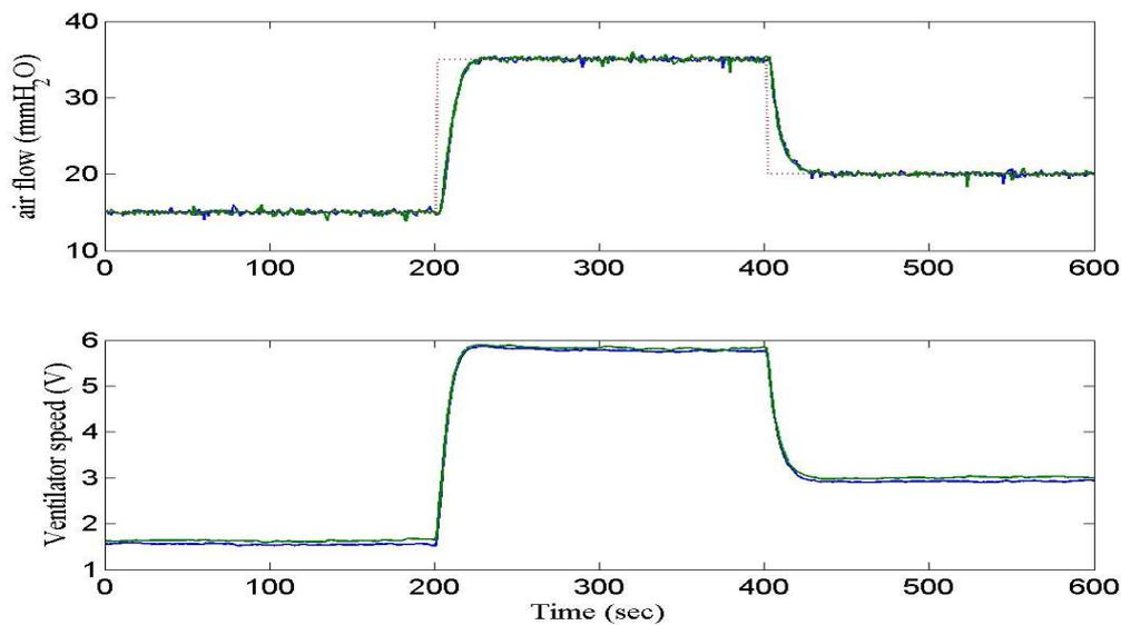
Figure 10: Top figure: closed-loop air flow response; bottom figure: Closed-loop ventilator speed control response. (Blue: Decentralized PI controller, Green: conventional PI controller, Red: set-point signal).
