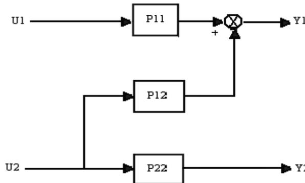
Figure 5: Partial interaction TITO Block diagram
