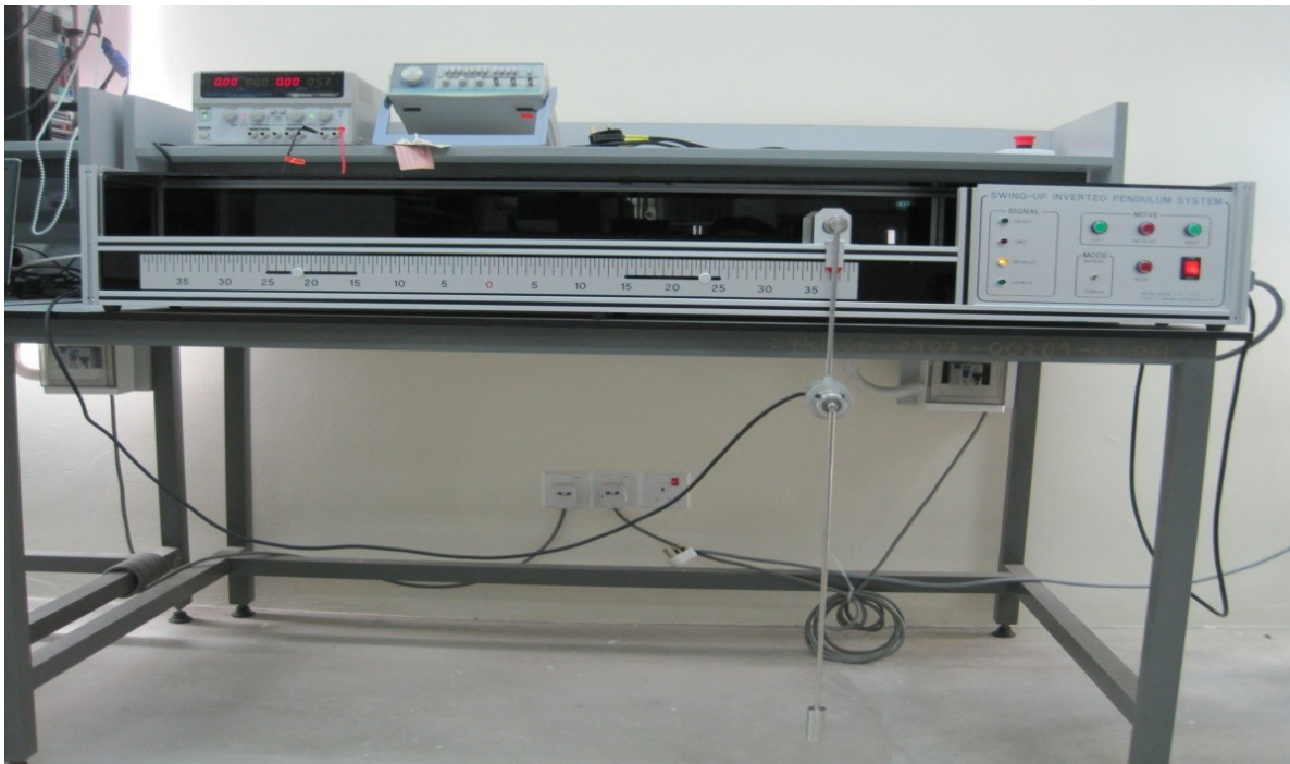
Figure 3. Double pendulum type overhead crane system at Control and Instrumentation Lab, UMP.
