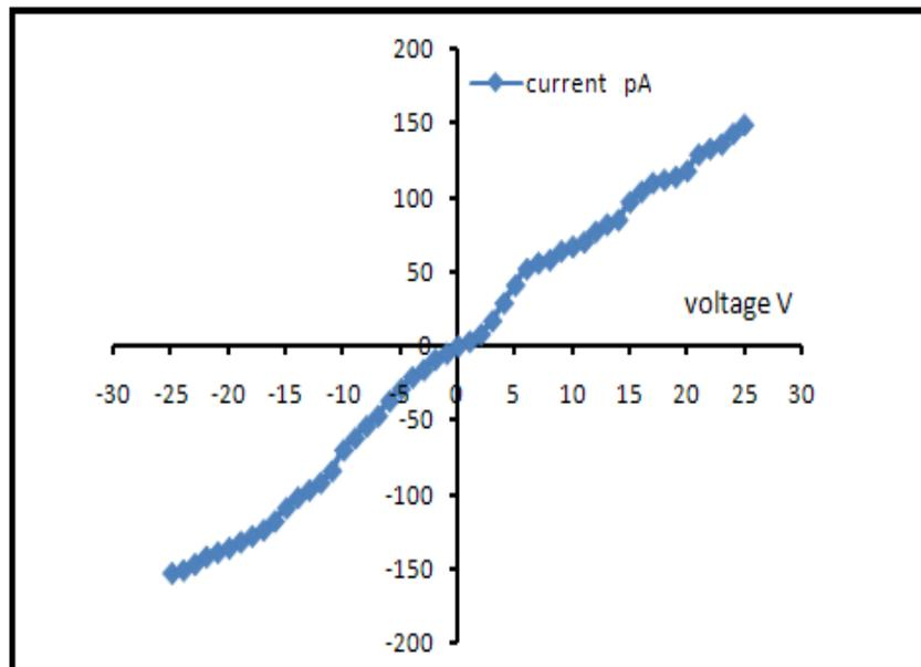
Figure 8. I-V characteristics of  $\text{Fe}_2\text{O}_3$  nanoparticles thick film.
