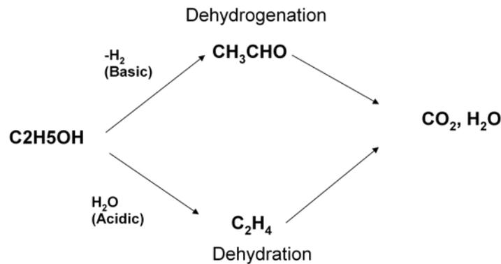
Figure 15. Routes of oxidization of ethanol vapor.
