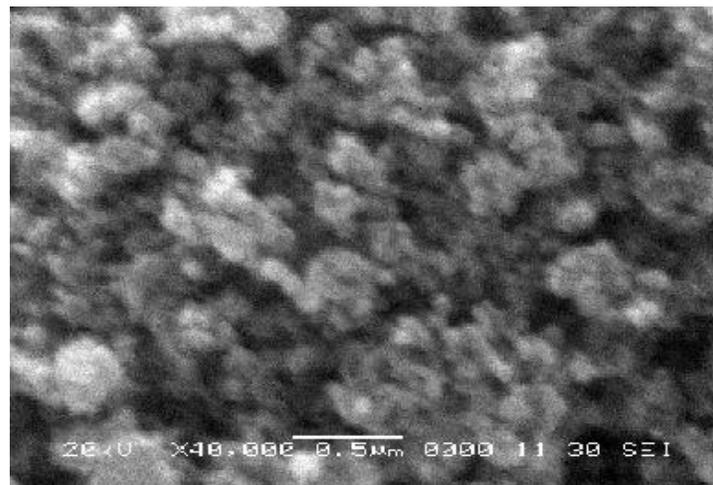
Figure 5. SEM image of the functional material nano Fe<sub>2</sub>O<sub>3</sub>.
