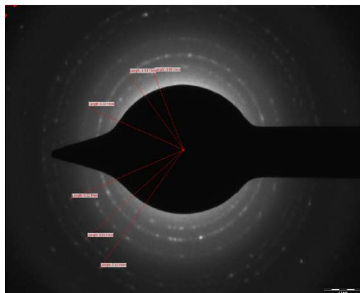
Figure 7. Selected area electron diffraction pattern of nano Fe<sub>2</sub>O<sub>3</sub>.
