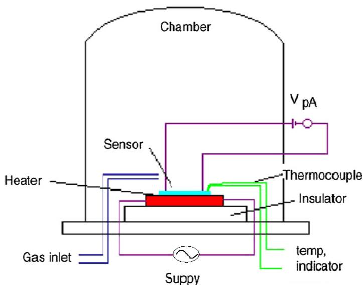
Figure 1. Schematic of static gas sensing system
