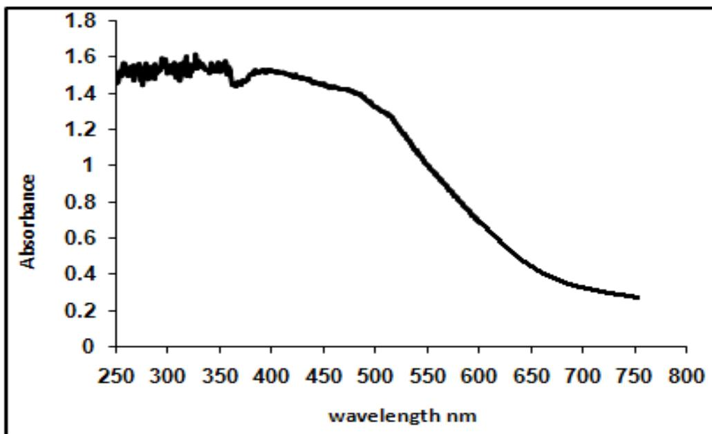
Figure 3. Optical absorbance of nano Fe<sub>2</sub>O<sub>3</sub> by UV spectroscopy.
