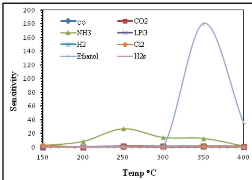
Figure 10. Sensitivity performance of nano Fe<sub>2</sub>O<sub>3</sub> film to all tested gases.
