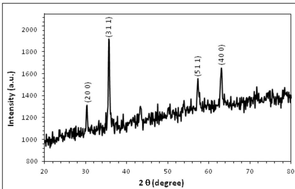
Figure 2. XRD image of nano Fe<sub>2</sub>O<sub>3</sub>.
