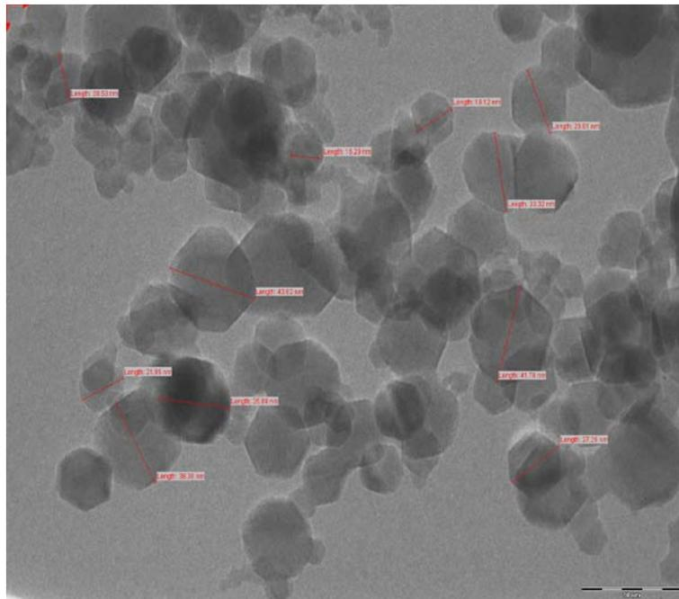
Figure 6. TEM image showing the nano sized particles of nano Fe<sub>2</sub>O<sub>3</sub>.
