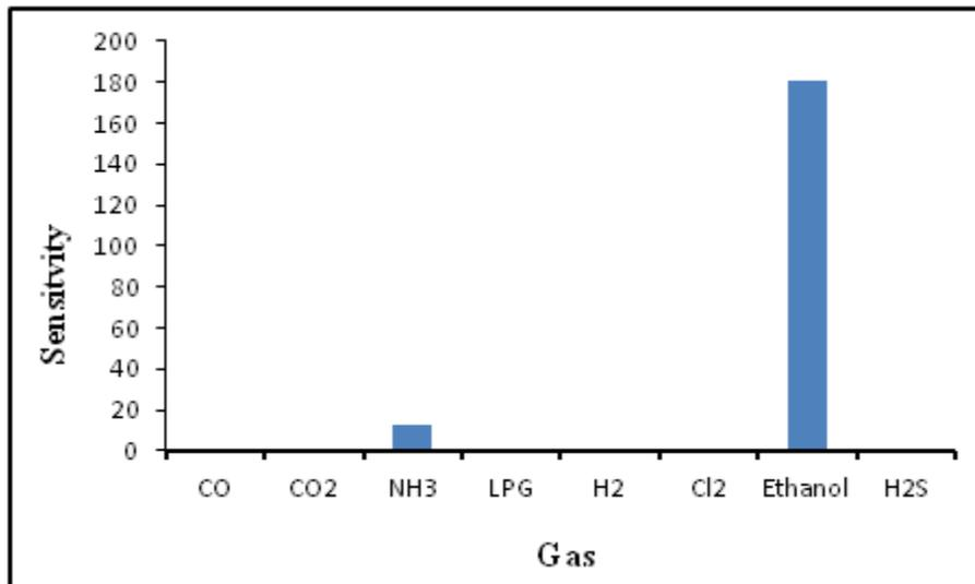
Figure 11. Selectivity to various gases at 350 °C.
