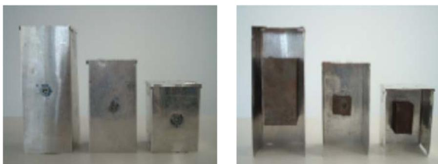
Figure. 2 Fronts and backs of different sizes of MLOs. The left photo, from left to right, shows the front sides of the large, medium and small MLOs respectively. The right photo, from left to right, shows their backs. The extra mass attached to the back of each object is also shown as examples. Extra mass helps change the weight keeping the front view unchanged.
