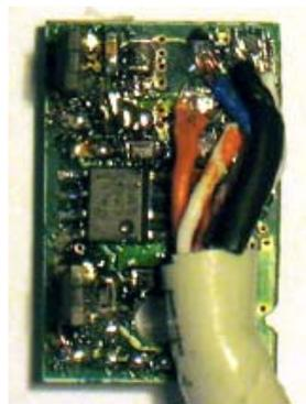
Figure 9. Experiment built Hall Effect sensor
