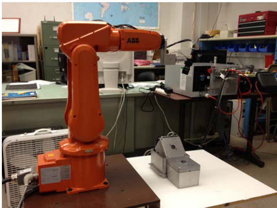
Figure 3. ABB IRB120 robot and the proposed calibration system
