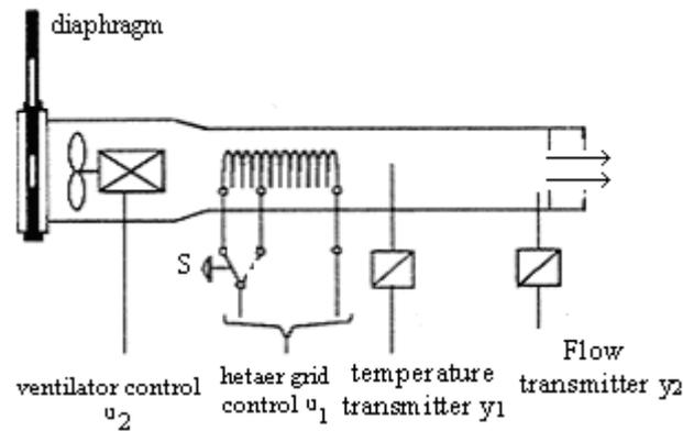
Figure 1. Schematic illustration of aerothermic process
