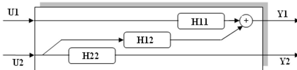
Figure 5: Schematic illustration of a partial interaction
