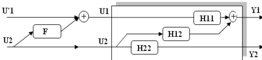
Figure 7: Decoupled system
