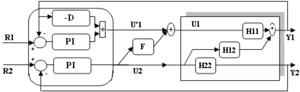
Figure 8. Block diagram of PI-D and PI applications
