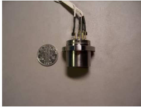
Figure 1. JSD-I/A quartz flexural accelerometer
