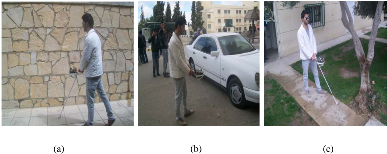
Figure 8: Testing the Smart Cane by a Volunteer in Terms of its Functionality. (a) Detection a Wall Using Sound and Vibration. (b) Detection Obstacles Below the Horizontal Level of the Smart Cane (c) Detection Obstacles while Turning the Smart Cane Left and Right.
