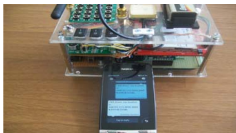
Figure 9: Testing GSM-GPS Module and Accelerometer Sensor.
