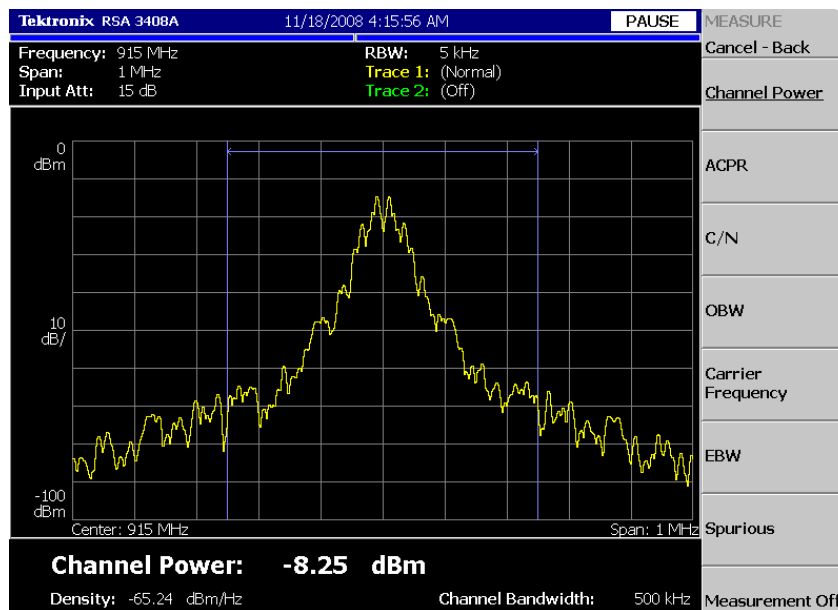
Figure 12. The spectrogram of RF transmission signal
