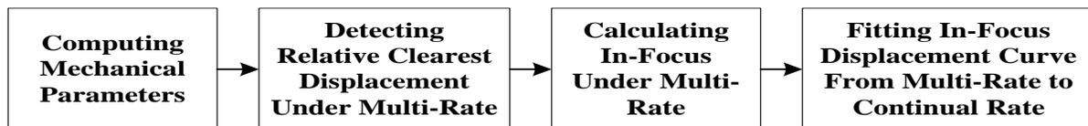
Figure 2. Block diagram of the proposed parfocality measurement method for a continuous zoom stereo microscope
