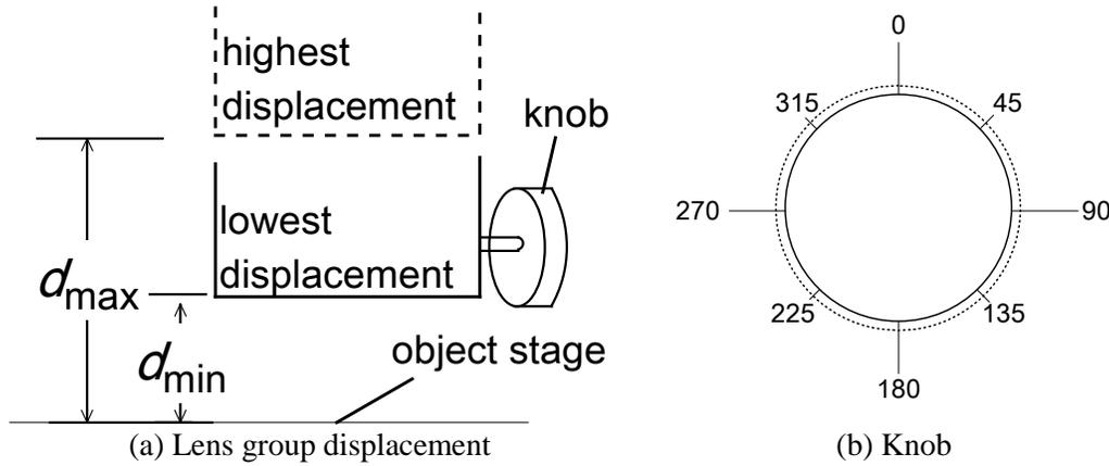
Figure 3. Mechanical structure of the object lens
