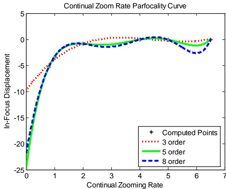
Figure 6. Continuous zoom rate parfocality curve
