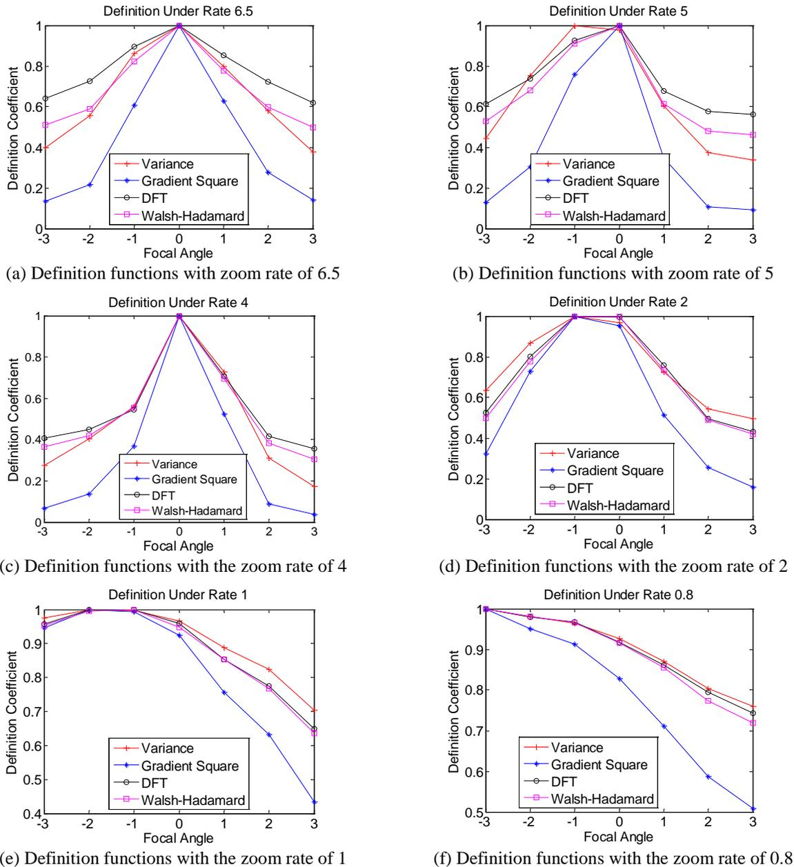
Figure 5. Definition function with different zoom rates
