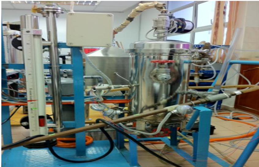
Figure 1. The hydro-diffusion essential oil extraction system
