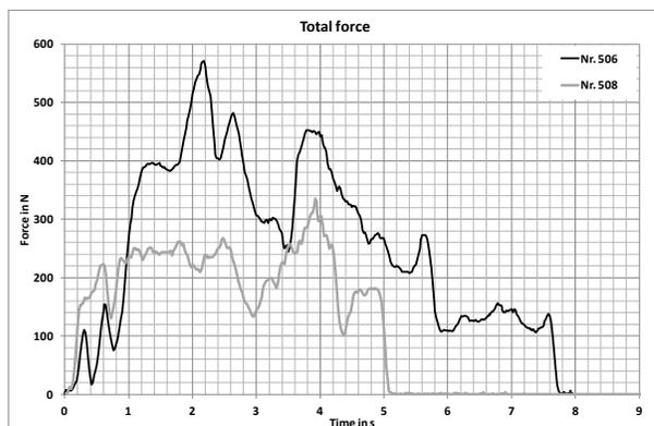
Figure 7 Total force of climber Nr. 506 and climber Nr. 508 exerted on the instrumented climbing hold.
