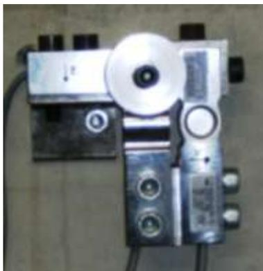
Figure 1 Orthogonally mounted load cells.
